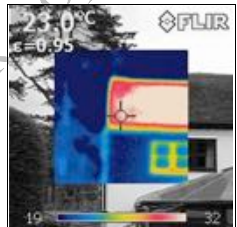
Cottage thermal image showing no roof insulation
