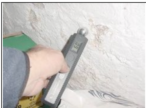
High damp readings in cellar
