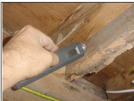
High damp metre readings on timber joists
