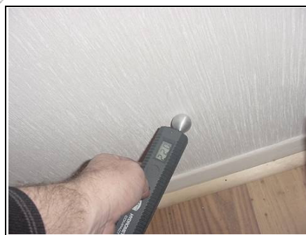
Testing for rising damp
