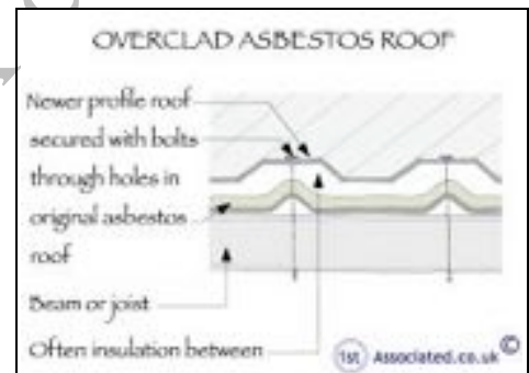
Overclad asbestos roof
