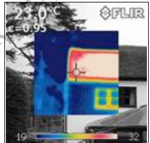
Cottage thermal image showing no roof insulation
