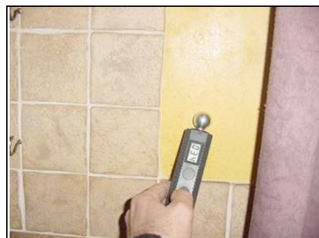
Testing for lateral dampness
