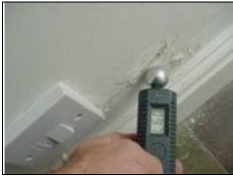
High damp readings of 97 in conservatory. They should be between 30 to 60
