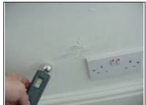
Obtaining high damp readings in the conservatory
