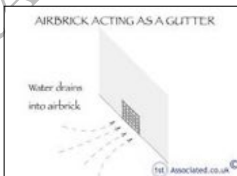
Airbrick acting as a gutter
