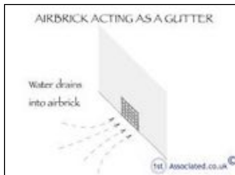
Airbrick acting as a gutter
