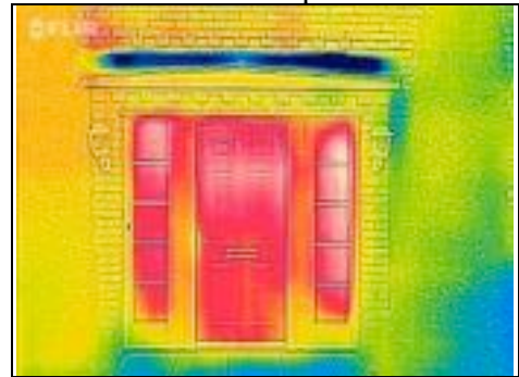
The front door from the outside showing heat from within on doors and windows, with the coolness to lead roof above entrance and paving in front of door
