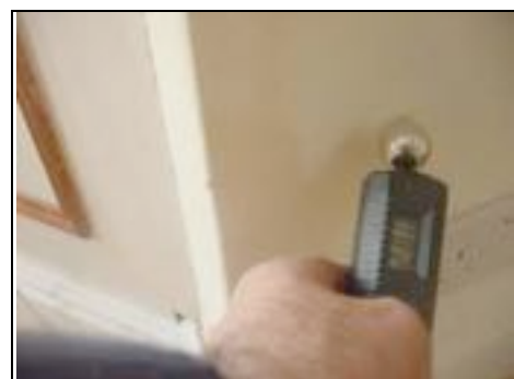
High damp meter reading to bay
