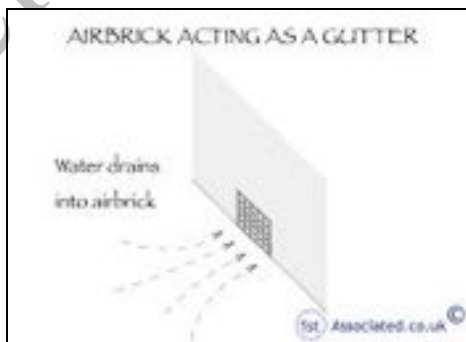
Airbrick acts as gutter
