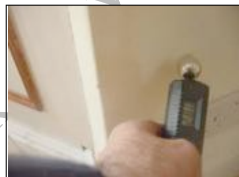
High damp meter reading to bay
