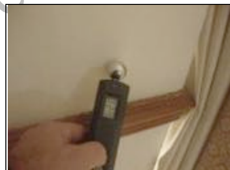
High damp reading of 62 Should be 30-60
